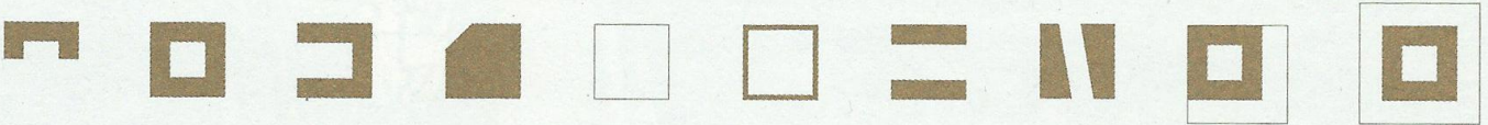
Figure ground diagrams (above) illustrating concept of carving social spaces out of the site, and a language of cutting, adding, filling, wrapping, slicing (below).
